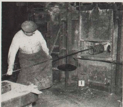
1—Edgar White tempering car springs in the fiery furnace.
