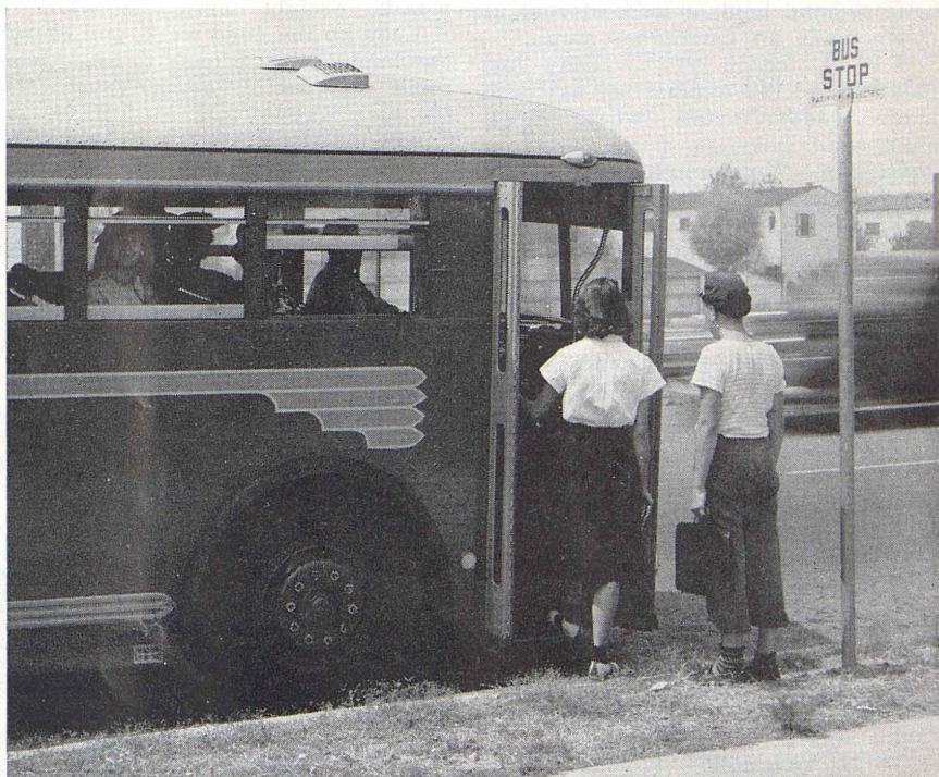
This picture indicates the proper position of motor coach steps in relation to the curb or landing when stopping for passengers to board or alight. When conditions do not permit stopping with steps close to the curb, coach should be stopped with steps 2½ or 3 feet from curb, or a sufficient distance so that passengers will be required to step down to pavement first and then to coach or curb, and in all such cases caution passengers to watch their step.
