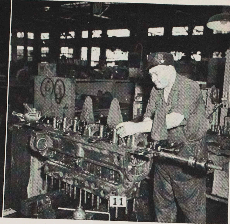
(11) AUGUSTUS FITZGERALD, Leader, is line-boring the main bearings on a 2100-class motor. Part of his job is to help the men—especially new men—out of difficulties with their work. (12) KENNETH CAMPBELL packs the rear main bearing on a White motor. (13) COVER PICTURE—DORIS SHULKEY is the sole woman at Torrance working as Auto Machinist. Before entering P. E. service on November 19, 1942, Doris used to run a service station at which her husband, Earl C. Shulkey (now Foreman of the Torrance Wiring Shop), did auto repair work. By helping him, she learned how to do her present work of overhauling valves. She does practically all the valve work for the Bus Motor Repair Section—refacing valves, tappets, valve seats, changing push-rod guides in the block, etc. The picture shows her grinding a valve on the valve-grinding machine. Mr. and Mrs. Shulkey have a married, 20-year-old son, Johnny, in the Coast Guard. Overseas for 12 months, he is now in Alaska wishing he were home with his wife and 15-month-old daughter. (14) STANLEY CARLETON installs a push-rod guide in a 1685-class motor block. (15) C. L. CROSS, Leader in diesel motor overhaul, reams a wrist pin.
