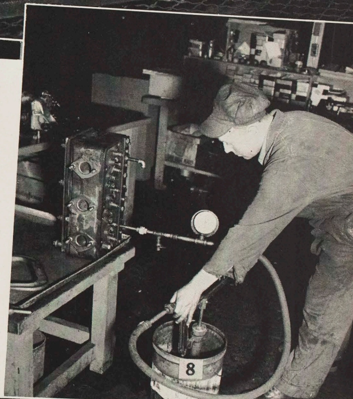
(6) REUBEN ("BARNEY") LOCK (left) and James Ogden are line-boring camshaft bearings on a Mack engine. (7) GEORGE WEINBERGER magnafluxes a Twin Coach crankshaft. Note the double strand of heavy electric cable around a section of the shaft. (8) ROBERT V. (BOB) SIMPSON water-tests a GMC cylinder head for cracks, using a hand pump to create 70 pounds of pressure. (9) BOB SIMPSON fits main bearings into a 1600-class motor. (10) C. J. BURNETT fits connecting rod bearings on a 2100-class crankshaft.
