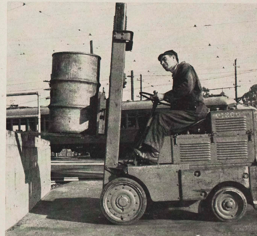
"NELLIE" is the title given to this useful electric lift truck. In service at Macy for several months, it has rapidly proved to be one of the handiest gadgets in the shops. Its electric lift will raise 4,000 pounds vertically 12 feet from the ground, and the lift will also tip its load slightly forward or backward at the touch of a lever. Nellie also saves labor by holding in place heavy appliances which must be fastened underneath cars. Store, Repair Shop, Garage, and Car House all use Nellie, who also has several sisters at Torrance.
