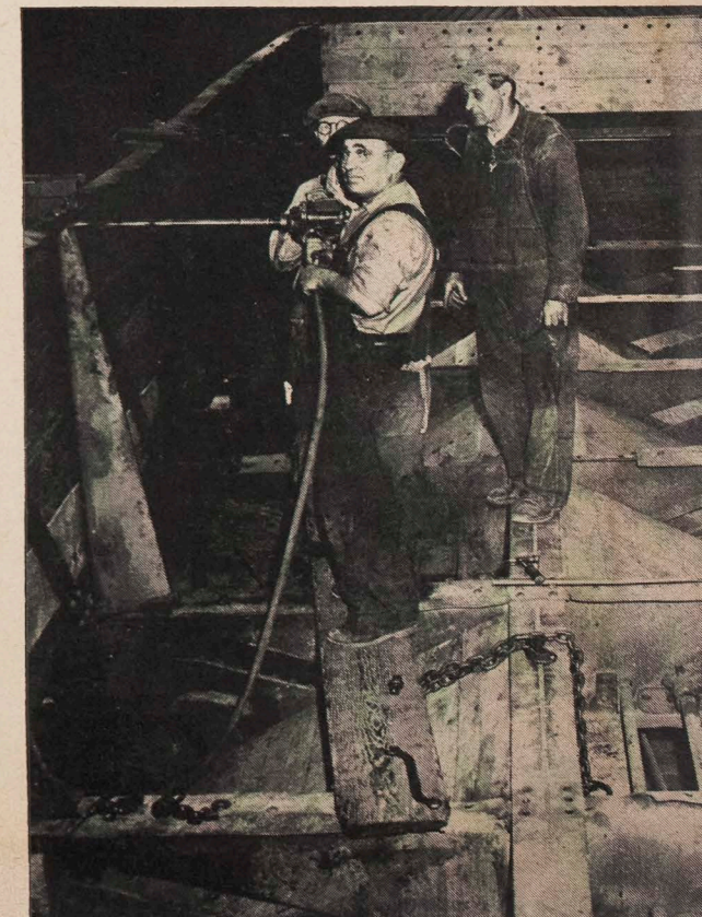
COVER PICTURE —Preparing to push in the bent steel framework at the end of a gondola are Car Repairers Leon Laubies (shoulder under bar), Frank W. Harlow (on horse), and Sam F. LoBue. The big jack is fastened to the end of the horizontal bar, which is attached to the coupler of the car. The men are placing against the end of the car one of two heavy steel arms also fastened to the jack. The whole arrangement (called a Stobo end straightener) forms a tripod. When the jack is raised, the only thing which can give way is the bent car end.
