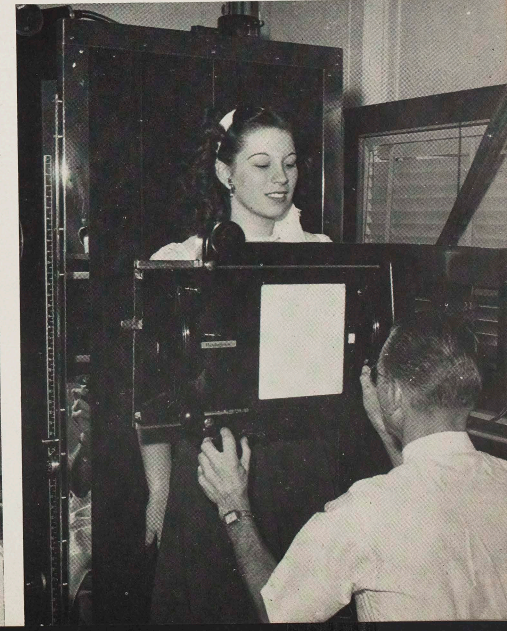
SPOT FILM DEVICE is demonstrated by Mr. Owen. The fluoroscopic screen is so arranged that at the touch of a button at his fingertip the screen instantly moves over, a film slides into place, and an exposure is made, for purposes of study and record, of the area seen in the fluoroscope.
