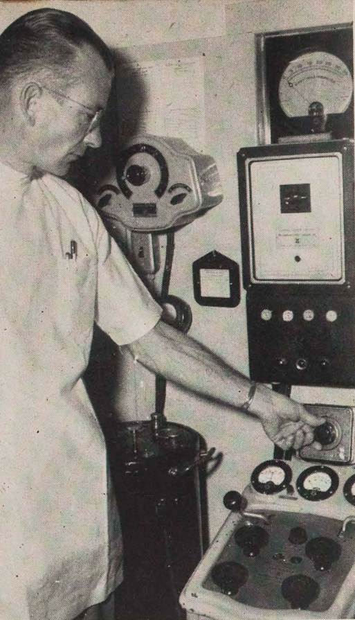
CONTROL SWITCHES AND DIALS for therapy and renovated radiographic machines. Mr. Owen shows how automatic timer is set for therapy control. Directly above timer is an automatic filter indicator which eliminates danger of X-ray overdose due to human error. Controls at left are for renovated radiographic machine.
