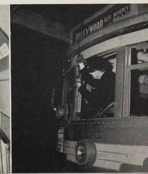
28. On turn-around, Dodge changes front trolley as Motorman changes rear one. Rear man changes others.
