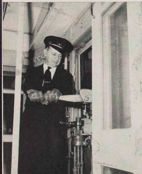
17. Since he's done all he could in advance, all he has to do is tighten hand-brake to tie car down.
