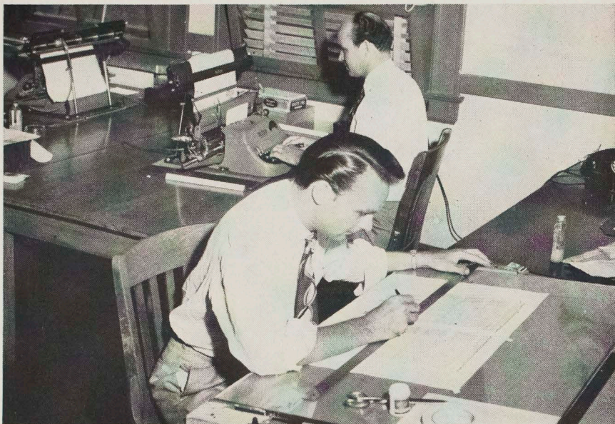
WHEN A SCHEDULE HAS FINALLY BEEN DRAWN UP AND APPROVED, it is set up on the vari-type machine and a layout is made. In this picture Jerry Vaughn, rear, is vari-typing, and Murphy Swindell is pasting in headlines and drawing in guide-lines for ease in reading. After the final layout has been checked for possible errors and approved, a plate is made and the schedule is finally run off on the multilith press in the Duplicating Bureau. Millions of copies of various schedules are thus run in the course of a year.
