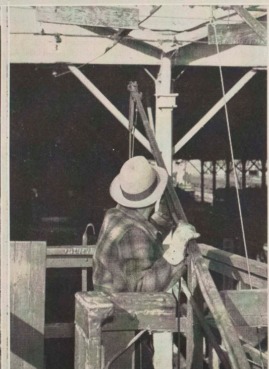
CONDUCTOR GOODMAN , in the tower of the car, shows how he places the greaser trolley against the trolley wire. Compressed air holds it up.
