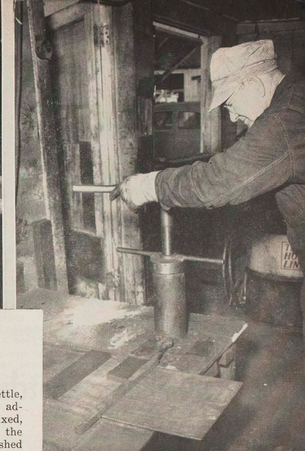
MAKING GREASE STICKS —Above, E. T. Johnston making a batch of grease at Washington St. Yard. At right, after mixture of graphite, paraffin, and grease has cooled somewhat, he puts some of it into the "gun" shown here, and by screwing down the piston forces the grease out of the bottom of the gun in the shape desired. He then cuts it off at the proper length, and repeats the process as necessary.
