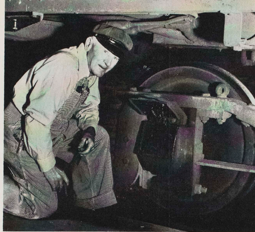
MR. FIXIT —Lee Merriman, Mechanical Department Leader on the Sixth and Main Viaduct and a PE man since 1919, inspects the journal box of a car. He goes around every car that comes in on his shift and repairs or reports any kind of trouble.
