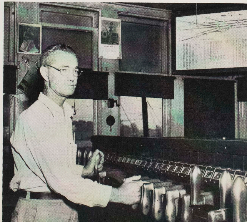
CONTROLS TRAINS —Paul G. Crunk, Towerman at Watts, estimates that he controls 250 train movements during his day-time shift from 7 to 3. All-electric Watts Tower controls the Torrance-El Segundo, Santa Ana, Long Beach, San Pedro, and Watts lines.
