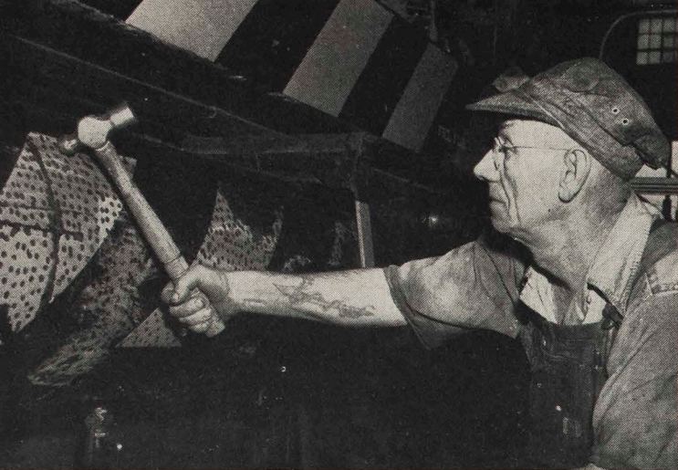
HAMMER TEST on air reservoir tank being demonstrated by Pipefitter Joseph Berdelle with ball-peen hammer. Actually, the test must be performed when tank is removed from locomotive.
