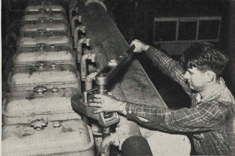
TORQUE WRENCH being used by Auto Machinist Robert Gish to tighten cylinder head stud nuts. Each and every bolt in the entire engine assembly is also subject to torque wrench test.
