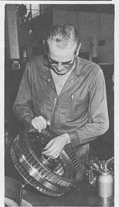
Norse C. Click, Mechanic "A", checks a rotor ring sleeve for wear.
