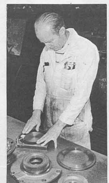
Charley W. Bauman, Mechanic "A" Leadman, checking a lined clutch disc on a 6200 class transmission.
