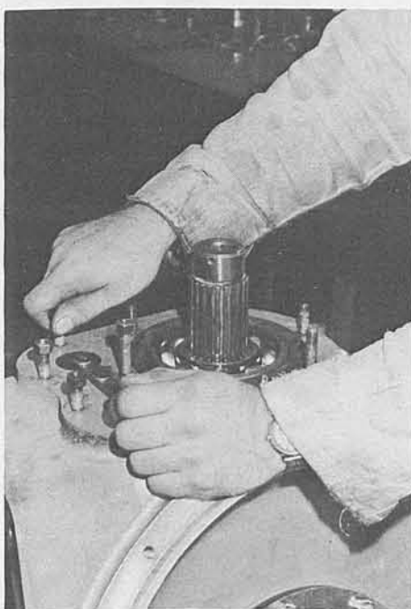
Removing the studs from the output end of a transmission.
