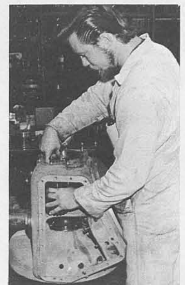
John B. Barber, Mechanic "B", ins'talls an idler gear in a 5100 class transmission.
