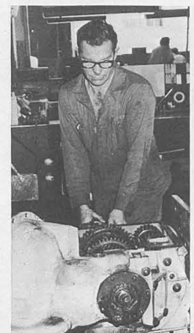
Dwayne F. Chisholm, Mechanic "A", removes a flange off a 5500 class transmission.
