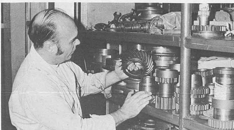
Charles J. Murrell, Mechanic "A", picks up a bevel gear from the parts shelf for use in a transmission he's working on.
