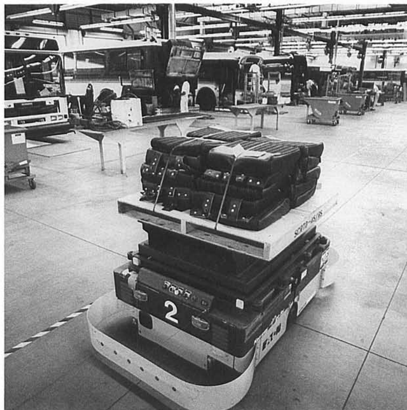
A beeping robot at work delivering parts at the MTA's Regional Rebuild Center.
