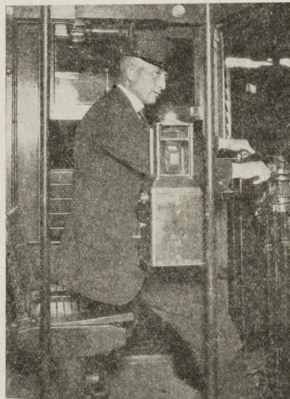
With the door closed the operator can devote his entire attention to running the car. This shows position of fare box and operating apparatus.
