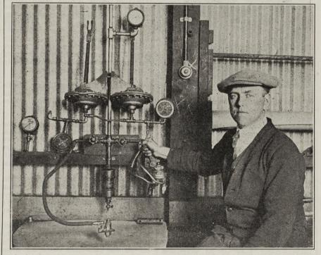
A NEW device, installed at the garage near Sixteenth and San Pedro streets, makes the adjusting of air brakes for the Los Angeles Railway busses an exact science and has eliminated all the guess work. Apparatus similar to the brake equipment on a bus, has been mounted on the wall. The valve which regulates the air pres-sure is attached, and set so that the gauge shows the right amount of air is being used. The valve is then re-
