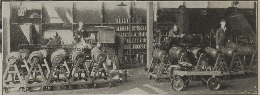
LOWER PICTURE: A BUSY CORNER OF THE TRUCK SHOP WHERE "C" INSPECTION, ARMATURE AND BEARING MACHINE WORK IS DONE. AT LEFT IS EMERY SAYER WITH HIS NEW LATHE; THOMAS FOWLER AND W. WELLER.
