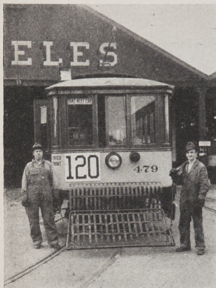
Left, John W. Knight and right, Warren H. Knowles, after completing the final inspection of the 120th and last car reconstructed from type "B" to type "BF" cars on our latest modernization program.
