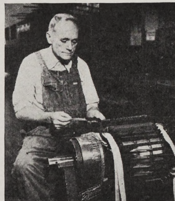
J. P. Hayes winding Westinghouse Type 514-L armature.
