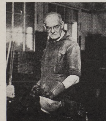
R. Smith pouring babbitt into axle bearing mould.
