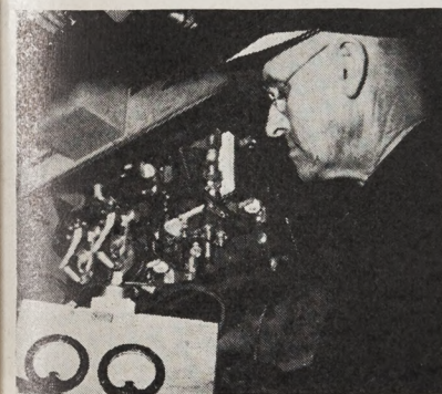
V. R. Bell calibrating voltage regulating panel, P.C.C. car.
