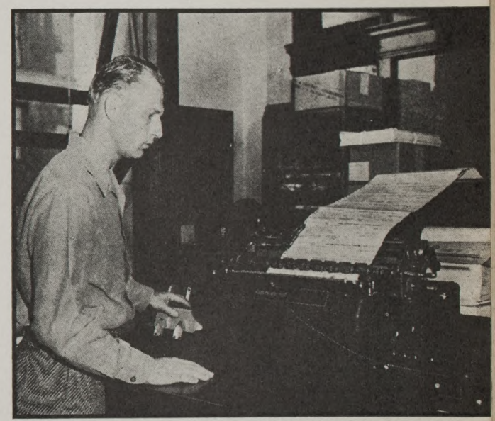
PAYROLL CHECKS are written by the printing tabulator as the three tabulating cards for each employe pass through the machine. The tabulator, operated by Jack Klemroth, is a combined adding, subtracting and printing machine.
