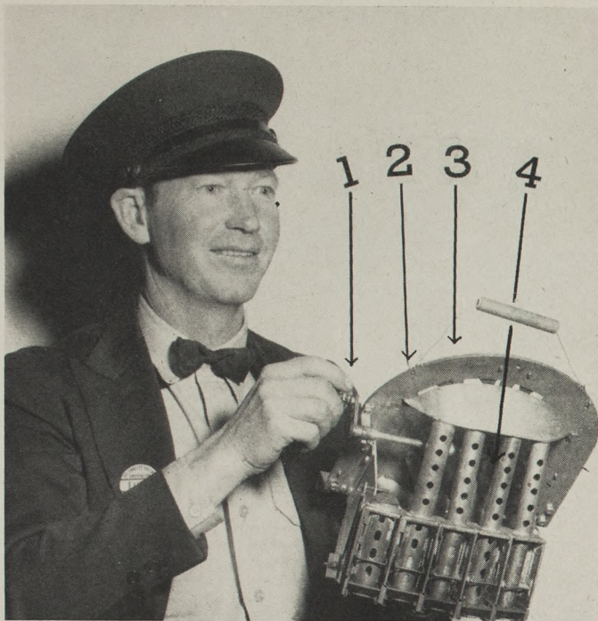
L. F. Beeson operates his changer by turning the crank (1) which revolves the flat wheel (2) causing the coins to go uphill and fall in slots (3). They drop in long changer barrels (4) that are ready for use.
