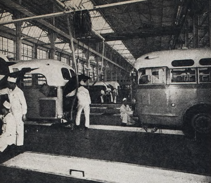
● Regular inspection at 16th Street. These mechanics go over coaches which pull in for inspection. Note the tubular suction ducts which carry the exhaust fumes from the muffler of the coach into the open air, making the Garage a fume-free work shop.
