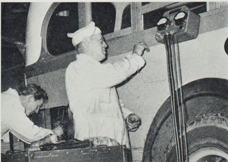
• Frequent testing of R.P.M. ratings, oil pressures, motor temperatures, and exhaust vapors foretell future failures.
