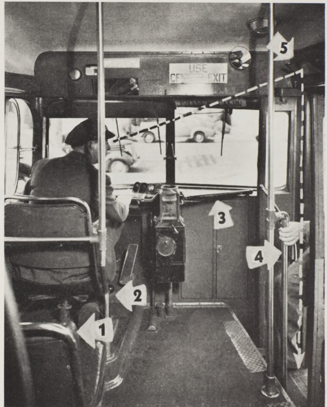
C • Five features are now being tested on the front end of the Guinea Pig Car. 1. A stanchion was removed from the first seat on the left hand side for the freedom of movement of the passengers. 2. The stanchion behind the operator was bent to give the passengers sitting in the first seat ample room to get in and out. 3. This angle bar has now been placed on all other P.C.C. vehicles. This prevents the passenger from leaning against the front windshield and obscuring the operator's vision. 4. This stanchion has been changed to make it easier and safer for boarding and alighting passengers. 5. New mirrors are being tested with which an operator can see the boarding or alighting passengers' feet by looking over their heads.
