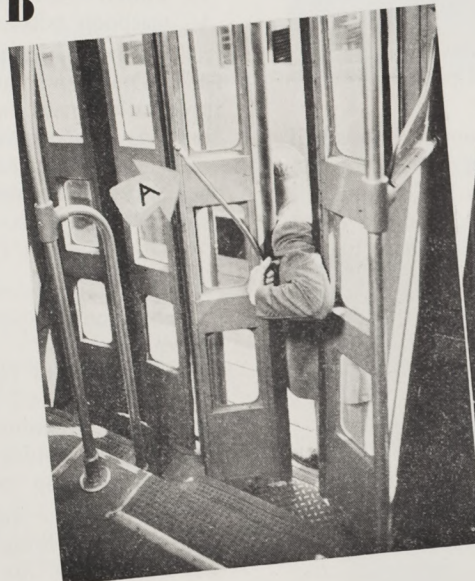
C • Five features are now being tested on the front end of the Guinea Pig Car. 1. A stanchion was removed from the first seat on the left hand side for the freedom of movement of the passengers. 2. The stanchion behind the operator was bent to give the passengers sitting in the first seat ample room to get in and out. 3. This angle bar has now been placed on all other P.C.C. vehicles. This prevents the passenger from leaning against the front windshield and obscuring the operator's vision. 4. This stanchion has been changed to make it easier and safer for boarding and alighting passengers. 5. New mirrors are being tested with which an operator can see the boarding or alighting passengers' feet by looking over their heads.
