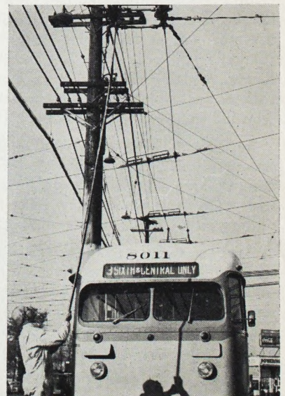
• Doing it the hard way is C. Canales, as he manipulates his pole in changing the trackless trolley switch points.
