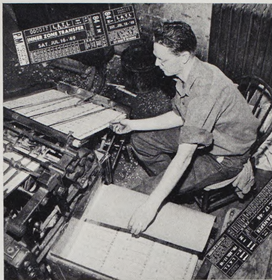
• Russell Parker takes the sheets of transfers off the press in bundles of 50 and places a cardboard backing between them.
