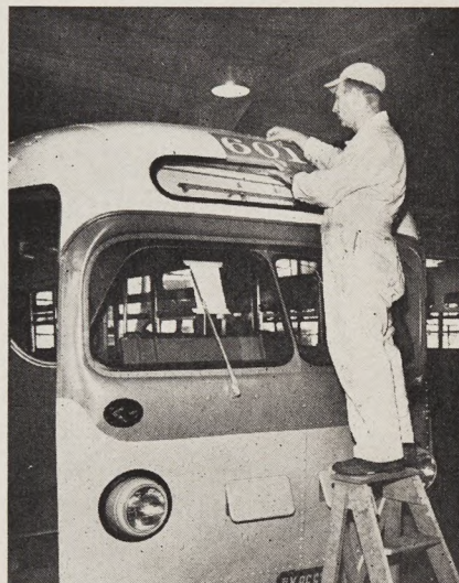
The thirty rebuilt coaches receive heaters built to fit in the space behind the fare-box. (Below) A completed job receives the last touch—Its number. Note how the windows have been slanted to conform with contours of modern design.
