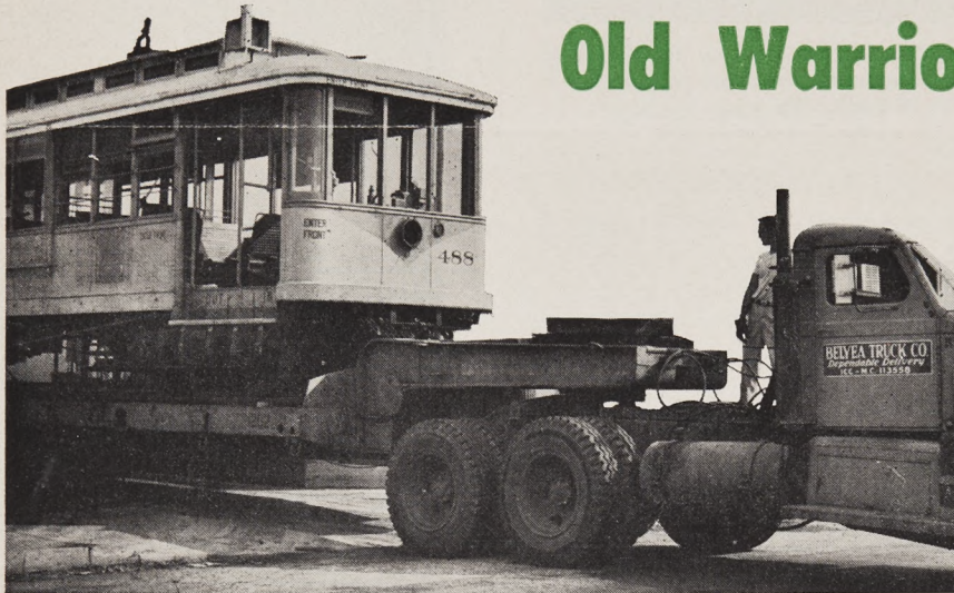
Old car No. 488 takes a last ride "piggy back" aboard a 22-wheel trailer-truck. (Right) Method by which street car is pulled up on bed of truck.
