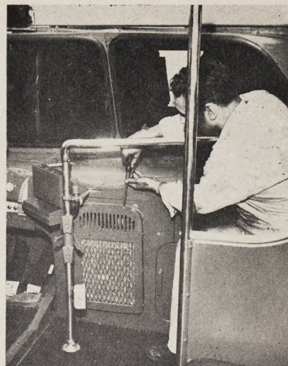
The thirty rebuilt coaches receive heaters built to fit in the space behind the fare-box. (Below) A completed job receives the last touch—Its number. Note how the windows have been slanted to conform with contours of modern design.
