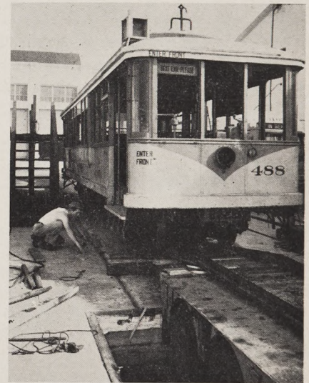
Old car No. 488 takes a last ride "piggy back" aboard a 22-wheel trailer-truck. (Right) Method by which street car is pulled up on bed of truck.
