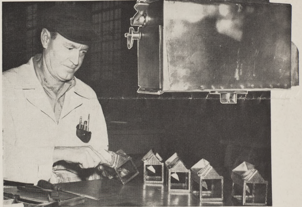
A close up of the collector's fare box. Art Rabey, of the sheet metal shop, assembles the first twelve to be built. More are in production to ease the load on traffic loaders.
