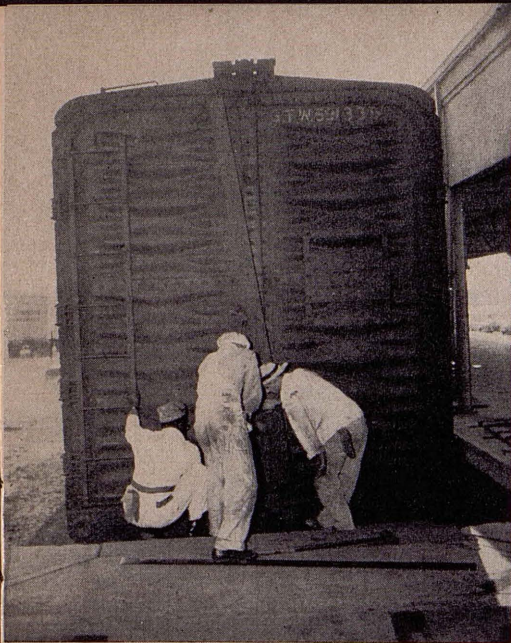
1. BUS ARRIVES in end-opening box car at SP auto dock, 748 S. Alameda. First job is unseal car doors.
