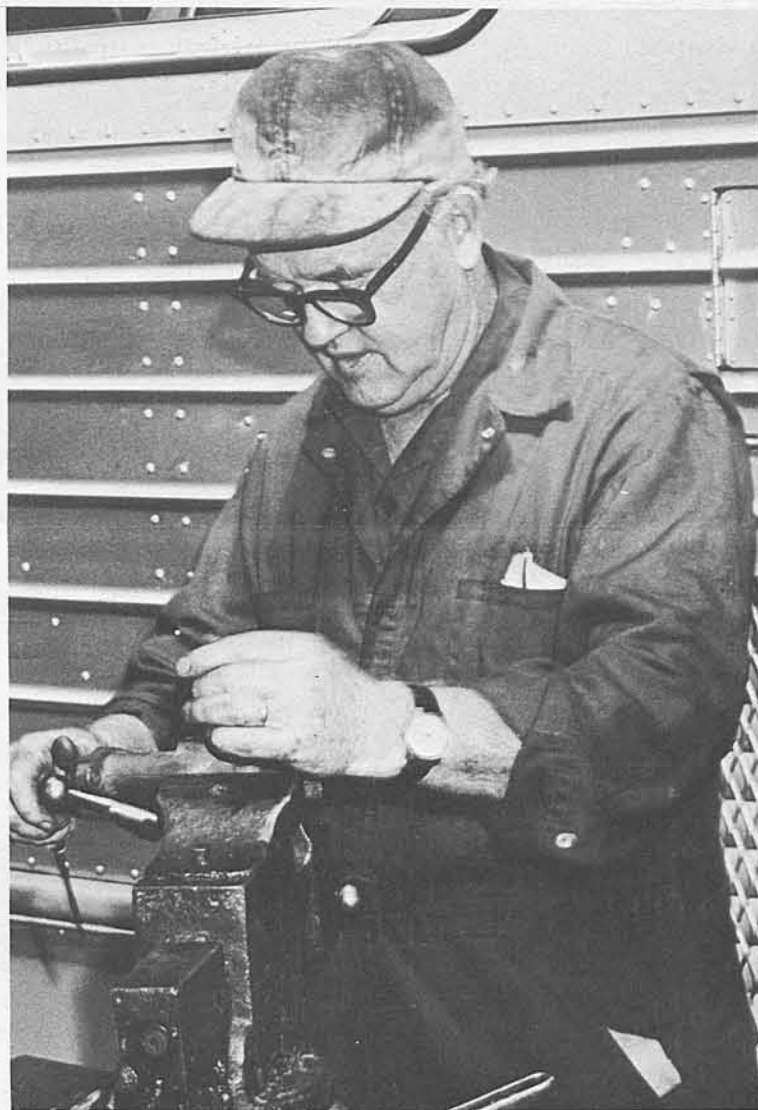
Ben Logan, mechanic "A" cleans carbon from the main air line of air compressor on bus behind him.
