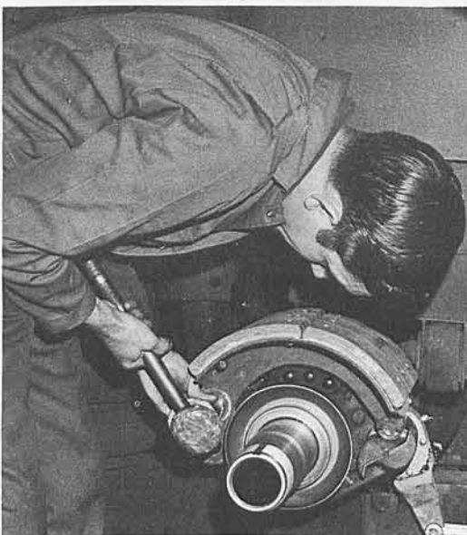
Bobby Bray, Mechanic "B", installs new brake shoes on rear axle.
