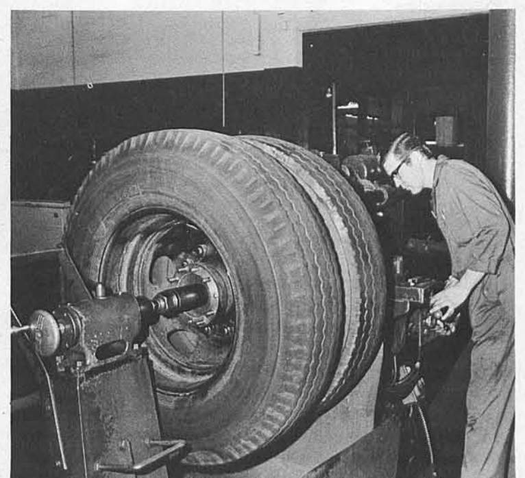
Everett Hunter, Mechanic "A", turns rear brake drum.
