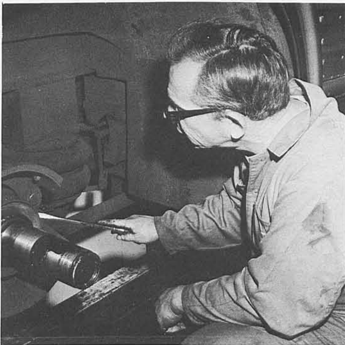
Joe Curtis, Mechanic "B", removes rear brake shoes.
