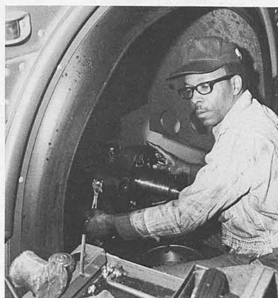
LeRoy Brown, Mechanic "A", replaces defective grease fitting on front brake assembly.
