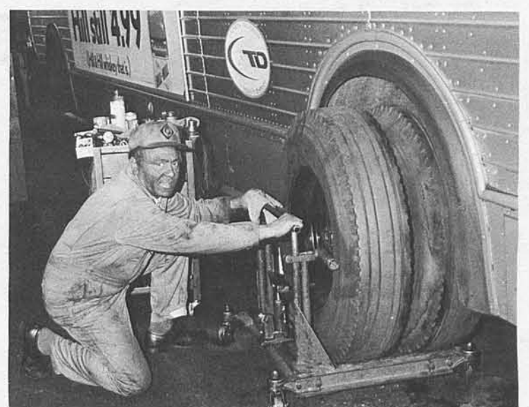
After new brake shoes have been installed, Harold Mouton, Mechanic "A", puts rear wheels back on.
