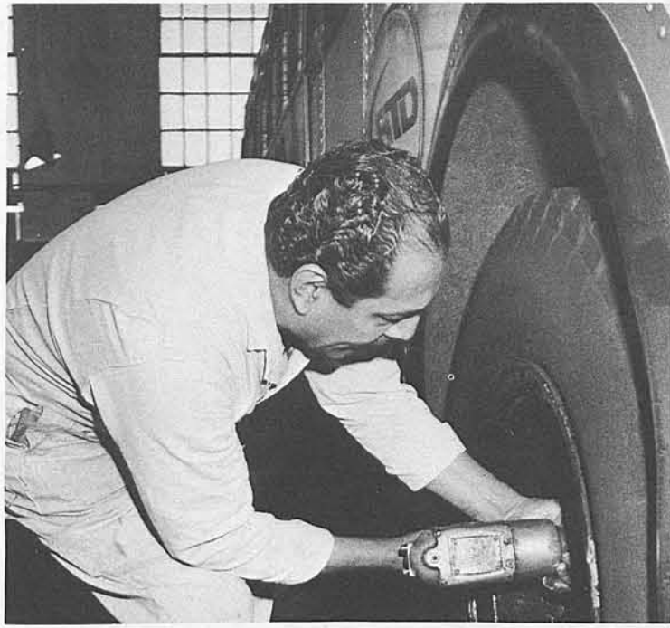
Joe Lara, Mechanic "A", removes rear axle shaft nuts. Axle must be pulled to remove rear wheels.
