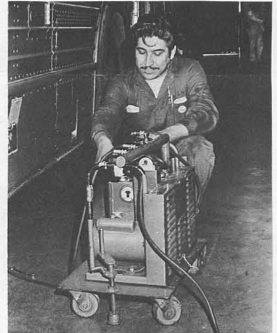
Bruno Falcon, Jr., Mechanic "A", uses vacuum to dry out air condition system.
