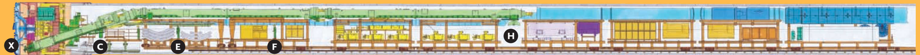
SECTION C Mid-Shield Screw conveyer (shown in green) removes soil from excavation chamber; air lock hatches (shown in blue) provide access to the cutterhead
