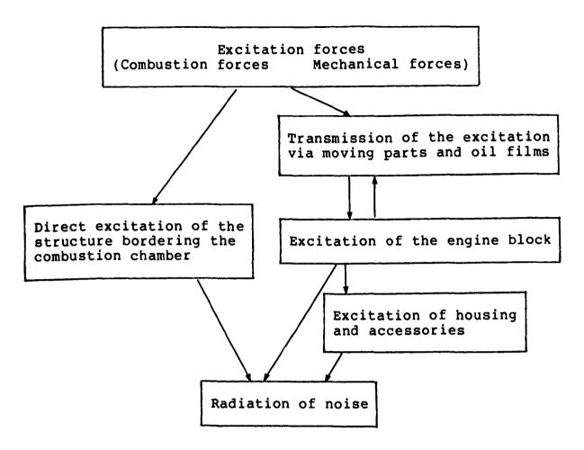
Thus the reduction of noise as a result of taking action on the engine itself can be concerned with the exciting force (explosion or combustion and the associated mechanical forces such as those due to side slap of the piston), with the transmission of that force via the moving parts and oil films or with the mechanical and acoustical response of the radiating structures involved (engine block, housing and accessories).
