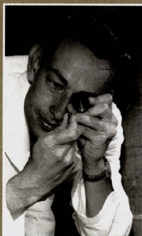
CONRAD VLECK LOOKS FOR OZONE-CAUSED CRACKS ON A RUBBER STRIP CIRCA 1960.
