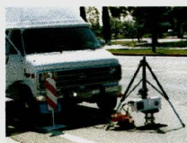
Smog Check II, including remote sensing of tailpipe emissions, tightens vehicle inspections.
