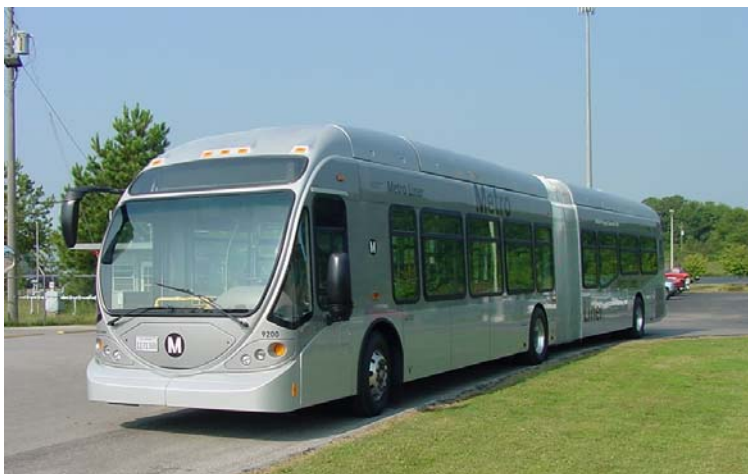
Low floor CNG-powered articulated vehicle for initial use on Orange Line
