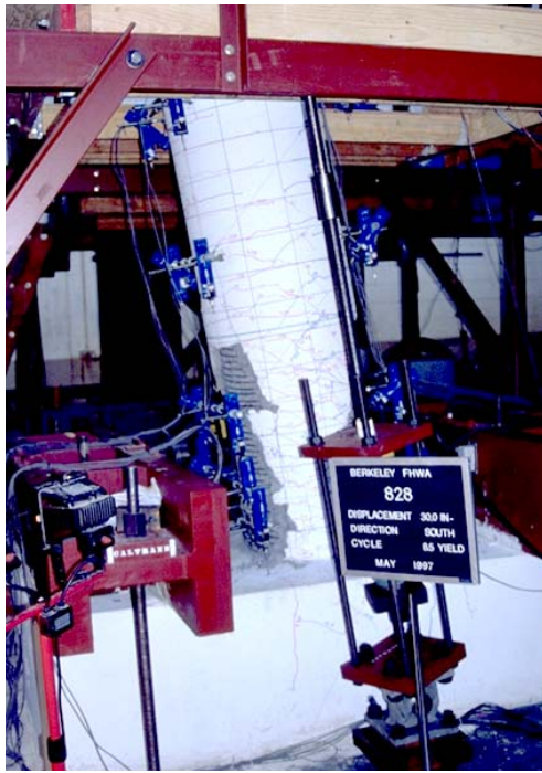
Figure 8-10. Laboratory test on a bridge column proves its toughness and its ability to undergo extreme earthquake movements.
