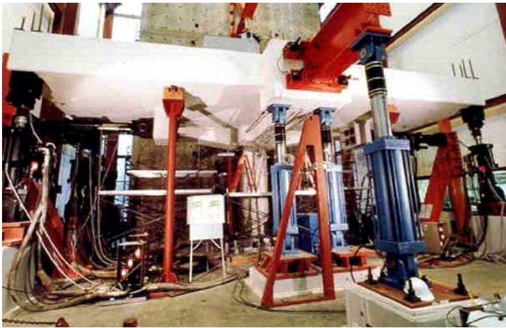
Figure 8-1. Half-scale proof-test model in support of the San Francisco double-deck viaduct retrofits.
