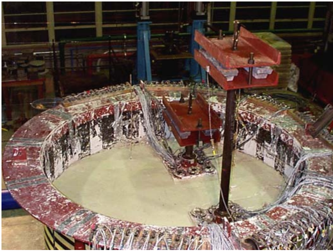
Figure 8-16. Tests of bridge foundation embedded in a large “bucket of mud” shaken by the earthquake simulator help engineers understand how to better design bridge foundations.
