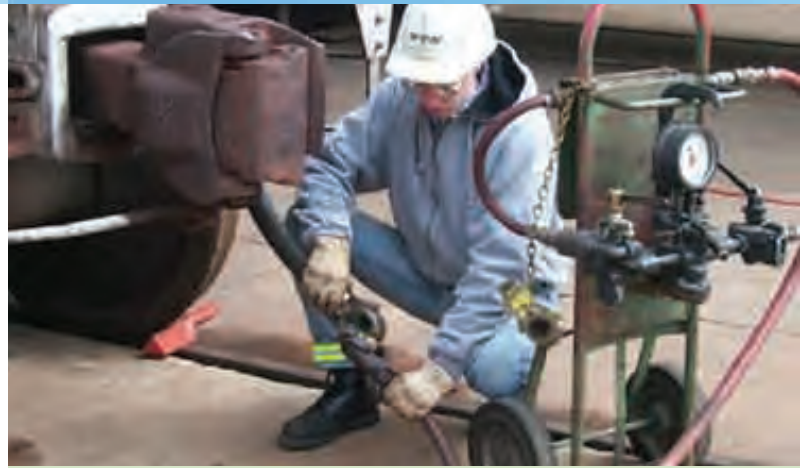
A TTX employee performs repairs on a coupling to help recondition a freight railcar.
