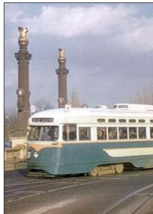
Figure 36: DC's original streetcar system operated in the L'Enfant Plan city without wires.
