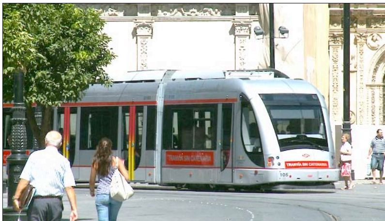
Figure 35: CAF Catenary-free streetcar (Photo Courtesy of Trainelec)
