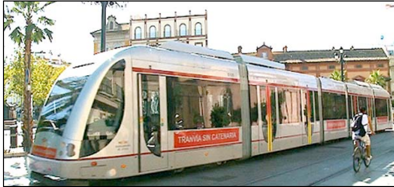
Figure 1: CAF Catenary-free streetcar (Photo Courtesy of Trainelec)
