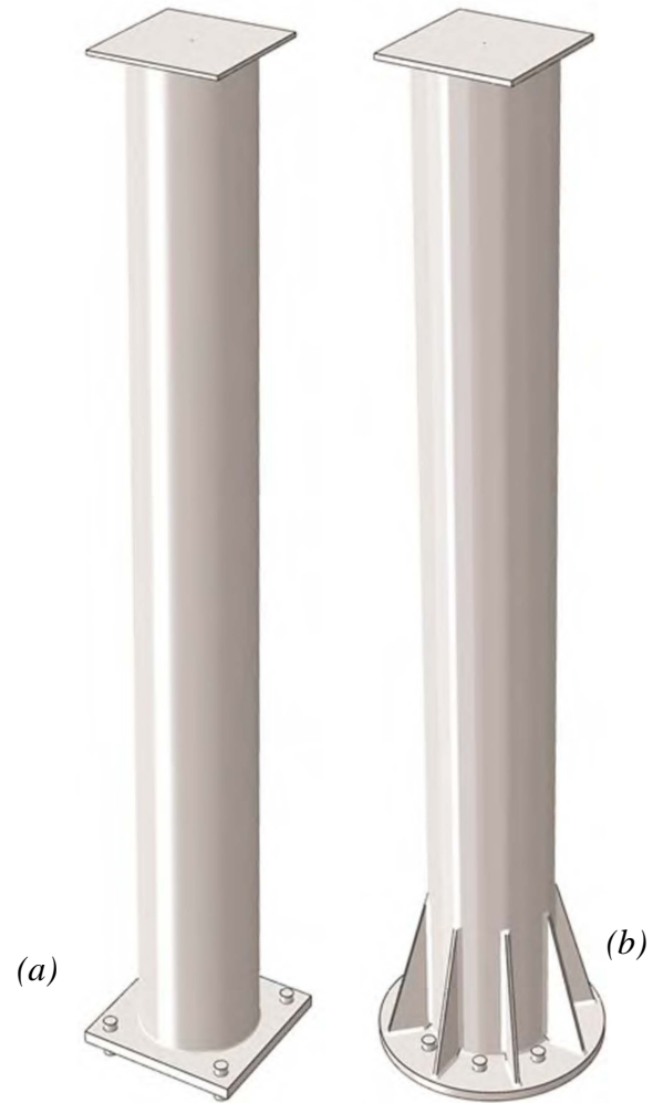
Figure 70 Global model of analyzed structures: (a) with unstiffened tube-to-transverse plate connection; (b) with stiffened tube-to-transverse plate connection
