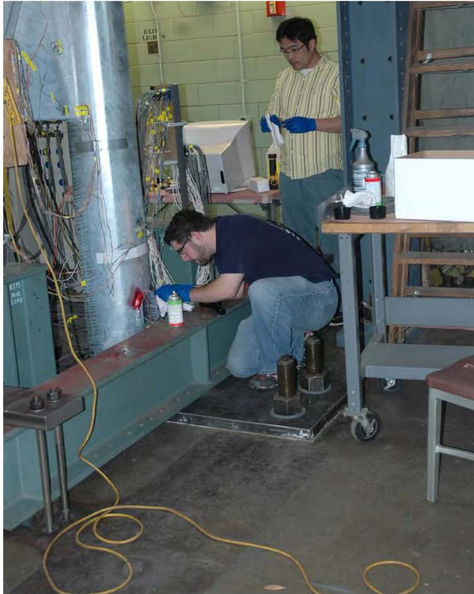
Figure 15 Hold down beam to reduce flexing of foundation plate
