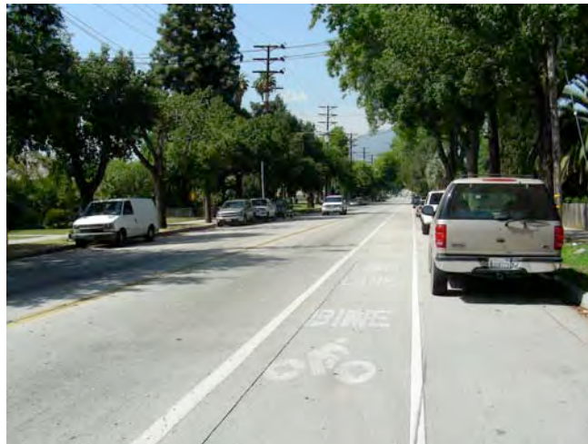
Figure 8-3: Bike Lane Striping and Stencil
