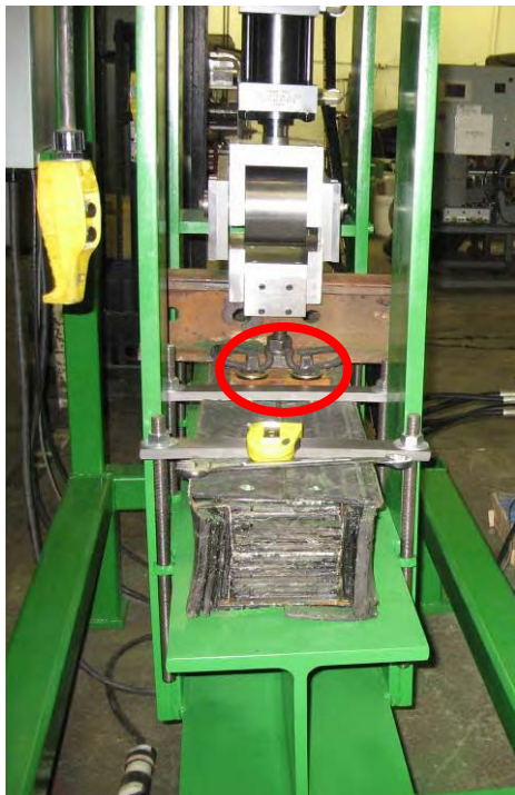
Figure 1: NP&G TireTie™ Lateral and 3-Point Bend Fixture
