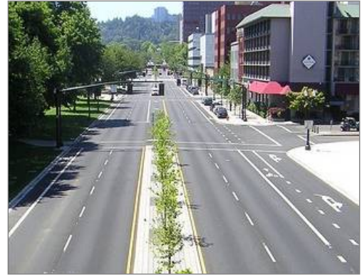
This street in Portland, Oregon previously had 13' lanes, which were narrowed to accommodate bike lanes without removing a lane.
