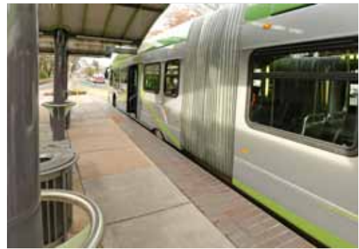
Eugene's EMX system provides level boarding from station to vehicle.
