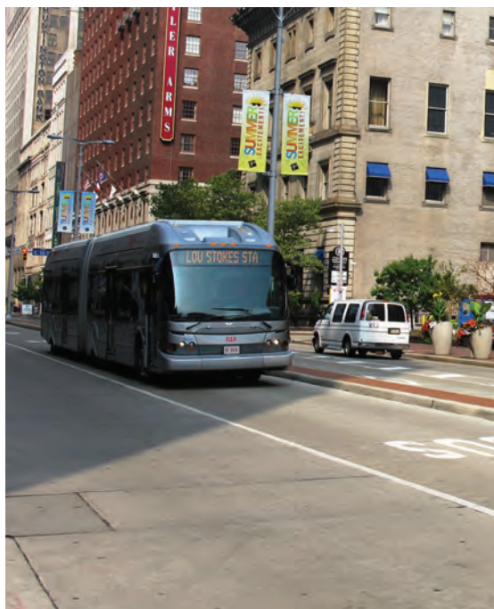
The Cleveland RTA was granted a design exception to allow eleven-foot bus lanes in order to fit their BRT into the existing right-of-way. Photo: Annie Weinstock, ITDP
