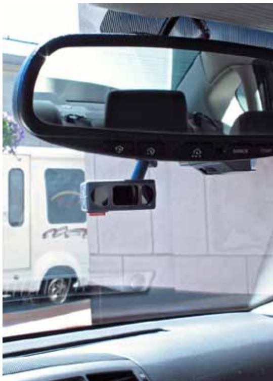
The SHRP 2 naturalistic driving study uses in-car sensors and cameras to collect data on driving behavior and crash risk. The study currently has more than 1,000 participants in six sites in the United States.
