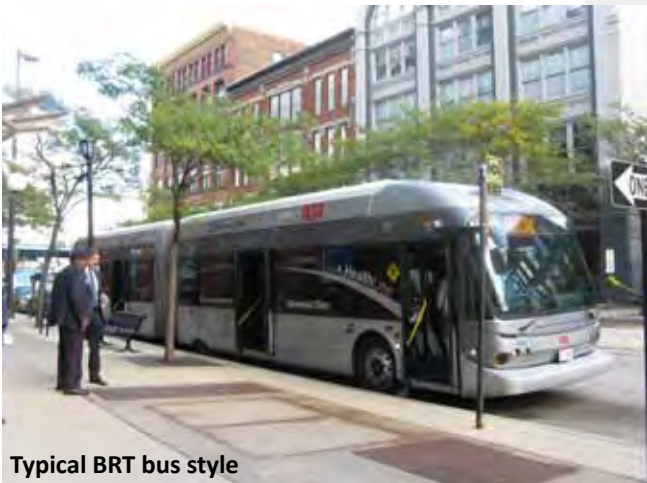
Multi-door boarding from platforms
