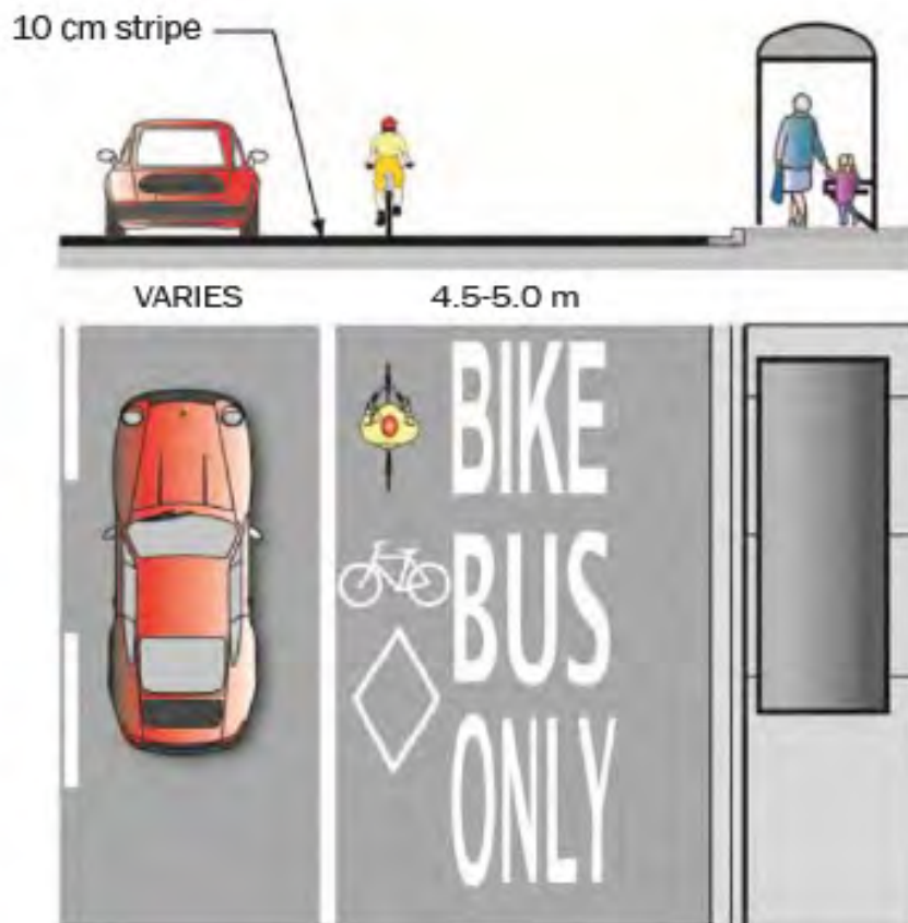
Figure 2.7 - Shared lane pavement markings (British Columbia)
