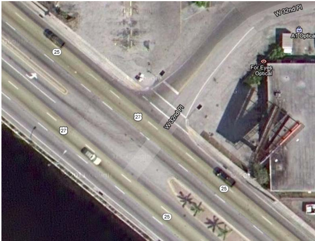
5-1(d) A full median opening with left-turn bay on only one direction.
