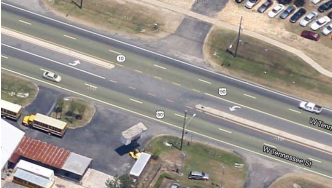
5-1(c) A full median opening with left-turn bays on both directions.
