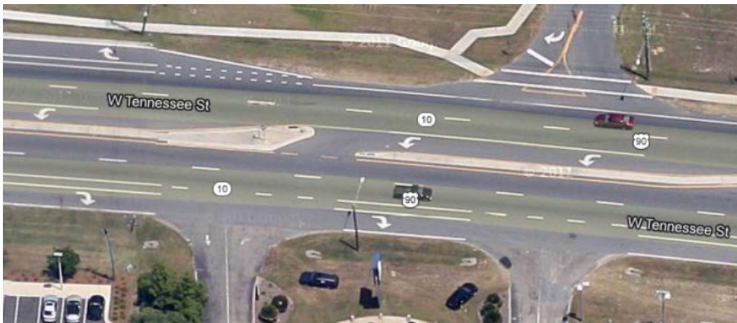
5-1(a) A uni-directional median opening.
