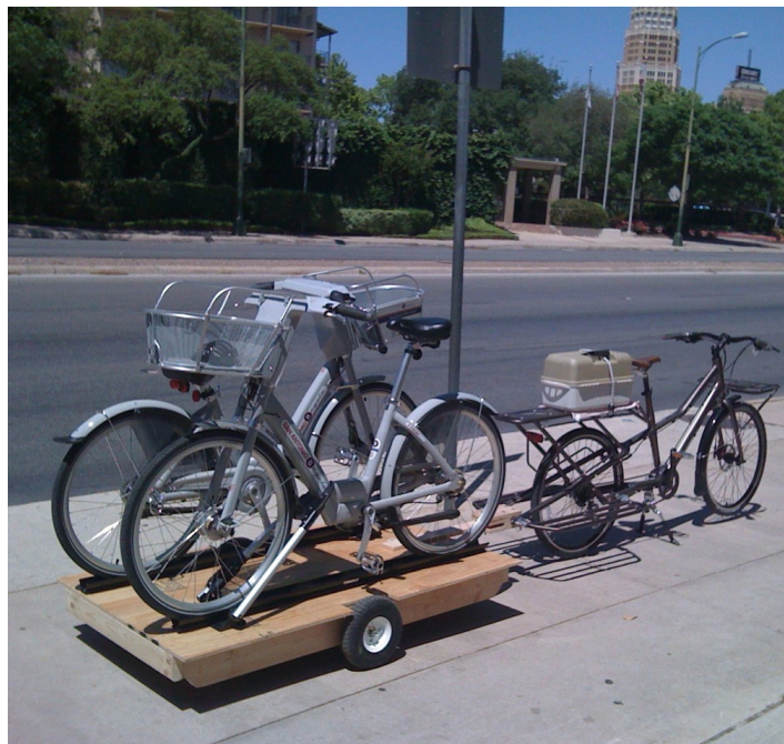
Figure 31: Bike powered trailer for bicycle redistribution Credit: San Antonio Bikes
