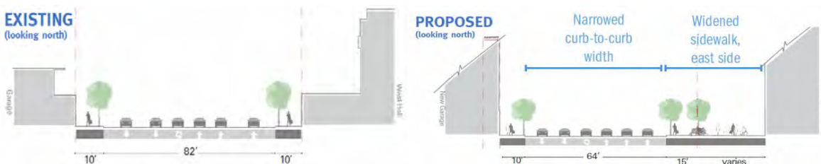
Figure 4: L.A. Live Way reconfiguration, looking north
